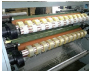
Slitting (cutting) Process (Converting machine+Packaging Machine)
